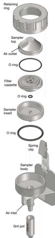
Figure 3. Configuration for plastic cyclone sampler and cassette
