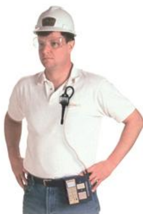
Figure 7. Cyclone sampler and pump on worker (© Copyright 2018 SKC Inc.)
